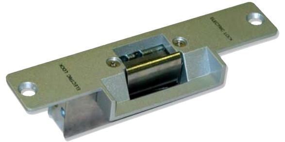
Ideal for use with the DIY Doorbell Video Intercom, the Swann Electric Door Strike allows you to open the door or gate with the touch of a button. The Swann Electric Door Strike is 12V operated and is fail secure so that it stays locked without power. Featuring a stainless steel faceplate and heavy-duty latch, the Swann Electric Door Strike will mount in most wood or aluminium frames.
